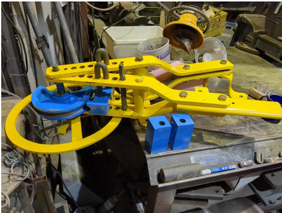
When bending heavy materials there is a long torque arm. It slides into the shaft of the arm that turns the die. I believe the holes are for an optional hydraulic ram.
